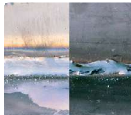
Descaled surfaces prior to welding lead to clean welding seams
