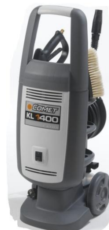
KL1400 Máquina Lavar com enrolador Classic 140 bar, 410Lt/H 2,0kW, 230V 2800 rpm
