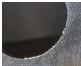
Before machining - Distinct burrs on the edge. Milling grooves on the surface.
